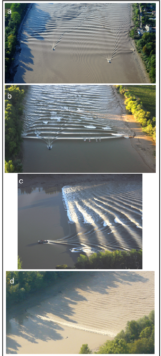
Fig. 3 Aerial photographs on the 10 th of September 2010 of the different mascaret types of the Garonne River. The Froude number increases from panel (a) to panel (d). a, Cambes, PK -16, 16h47 UT; b, Podensac field site, PK -32, 17:31 UT; c, Pont de Beguey, PK -33, 17:37 UT; d, east Arcins river branch, PK -6, 16:15 UT.
